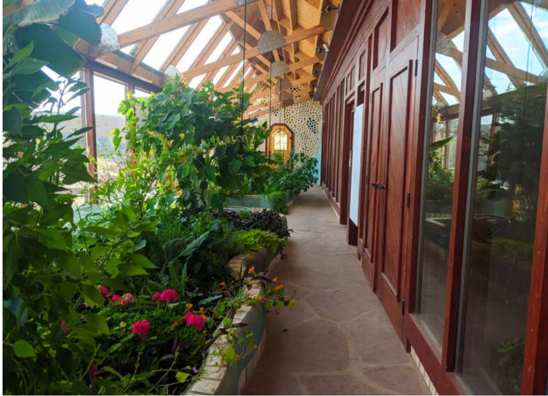
Good as green. Plants throughout the Earthship provide food, filtered graywater for toilets, and cleaner indoor air. CREDIT: MEREDITH ALBURY/EARTHSHIP BIOTECHTURE
