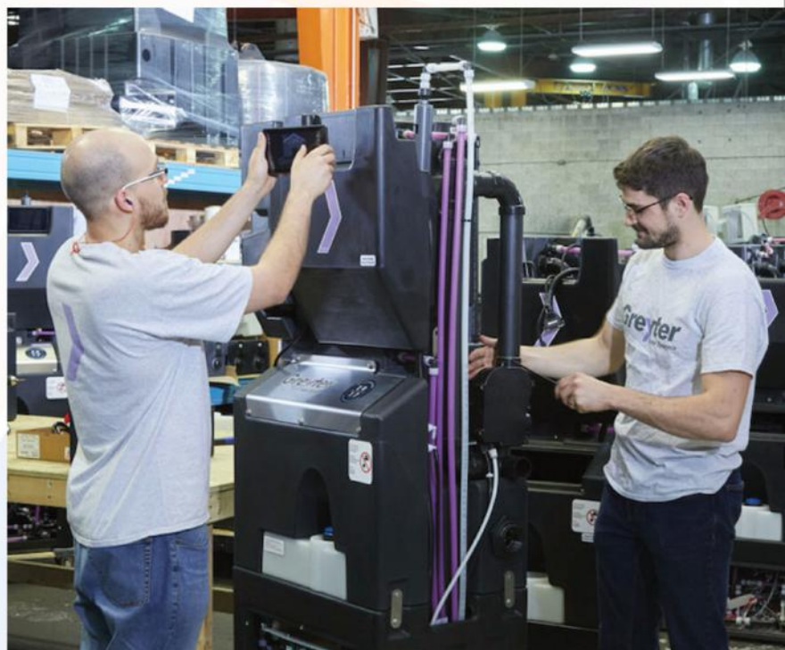
Continuous flow. Greywater collection units such as the Greyter HOME Water Recycling System provide an easy way to efficiently repurpose shower and bathtub runoff. CREDIT: COURTESY OF GREYTER WATER SYSTEMS
