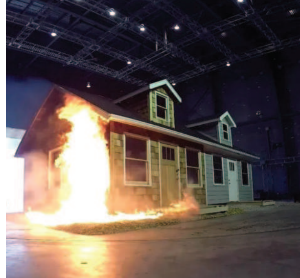
Combustible challenge. A resistance test in 2024 revealed that a shed built to 1980s standards (left) can't hold up to a fire, while one constructed under 2008 standards (right) isn't harmed.
