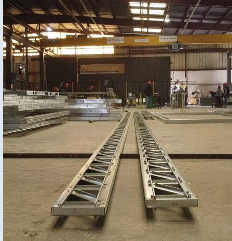
Anti-carbon construction. The steel foundation for a Dvele home has 80 percent less embedded carbon than concrete. CREDIT: GARY HORBACH/DVELE
