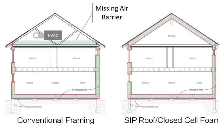
Figure 2: This redline air barrier test shows a missing air barrier at the top side of attic insulation in a vented attic.
