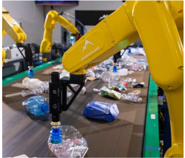
A 'sorted' effort. EverestLabs' robotic sorter uses AI to identify recyclables from regular waste on an assembly line—a far more efficient process compared to human hands. CREDIT: COURTESY OF EVERESTLABS
