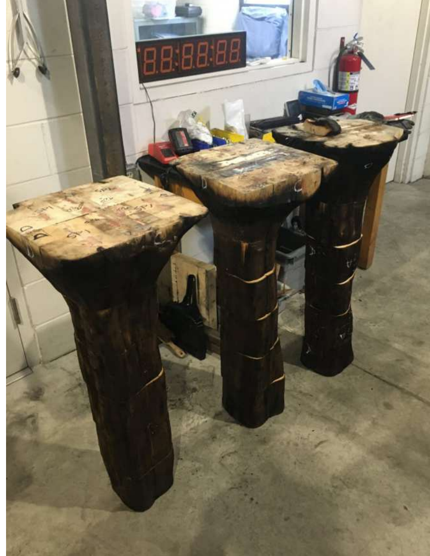
The fire inside. A three-hour burn test revealed that mass timber's outer structure can slowly incinerate, but the interior remains undamaged. CREDIT: COURTESY OF KORB ARCHITECTURE
